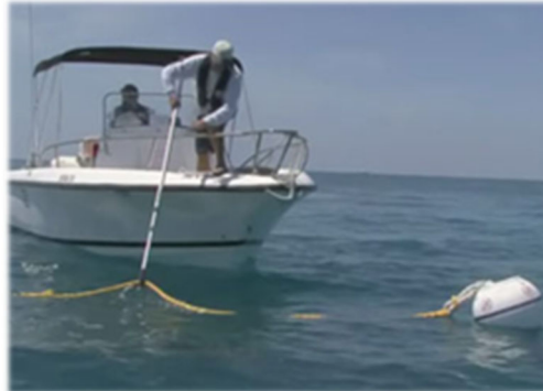
Figure 2-42. A boater secures the buoy mooring line to anchor his vessel. Source: NOAA
