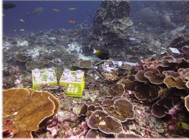
Figure 2-7. Short-term and long-term moored instruments deployed at Jarvis Island by the NOAA Pacific Islands Fisheries Science Center. The yellow crates are the temporary deployment (1-3 days) of water sampling units) and the CTD and pH sensors (in the metal cage). The Calcification Accretion Unit and an Autonomous Reef Monitoring Structure (the square structures) toward the right in the photo are the longer-term deployments (~3 yrs). Source: NOAA Pacific Island Fisheries Science Center
